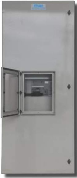
Figure 4: 1.3MW, 480V, 2000A Generator Disconnect & Output Protection Molded Case Circuit Breaker NEMA 1 Enclosure with Window Kit
