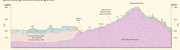
Schematic north-south cross section through the Post Falls quadrangle from the Rathbun Plateau (north) to the Blossom Mountain uplands (south) demonstrates the stratigraphic and topographic relationships of surficial units. Not to scale.
