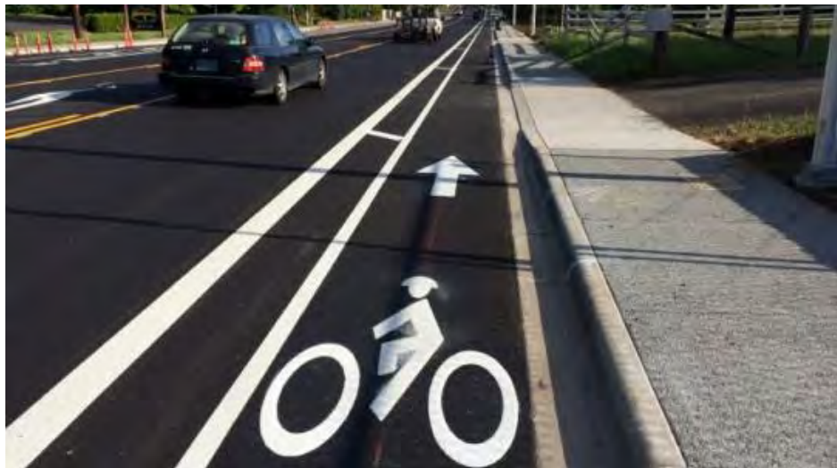
Figure 8-8. Buffered Bicycle Lane
